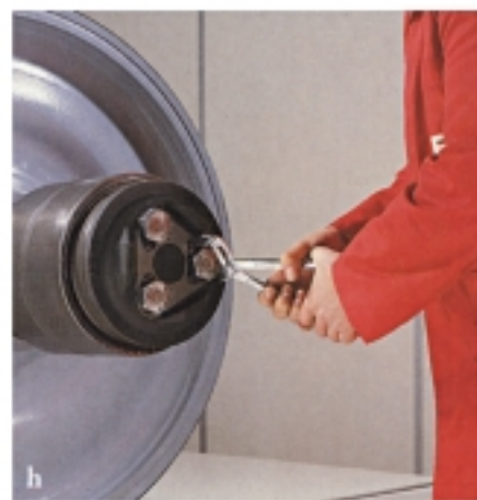
Tightening torque for the end cap bolts for TAROL units in metric dimensions
