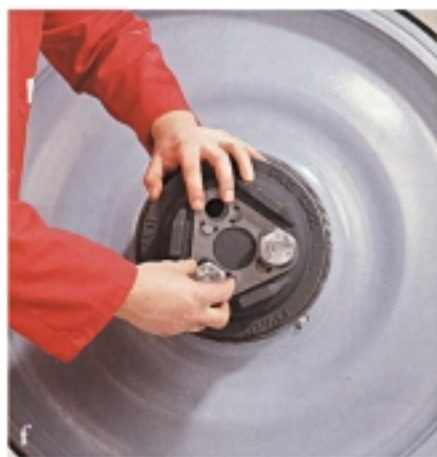
Tightening torque for the end cap bolts for TAROL units in metric dimensions
