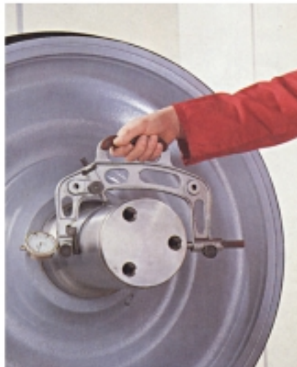
Device with three pins for checking the pitch circle diameter and the parallelism of the fastening holes at the face of the axle journal
