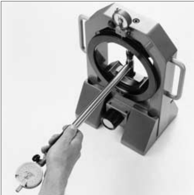
76: The measured raceway diameter is transmitted to the boundary circle measuring instrument with the aid of an internal dial gauge. The boundary circle measuring instrument FAG MGA 31 is used for cylindrical roller bearings with separable outer ring, such as FAG NN30ASK.
