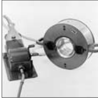
45: Induction coil for 380 V with bearing inner ring
