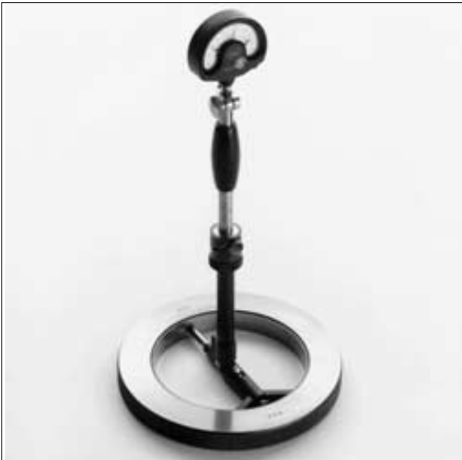
5: Comparative measuring instruments are especially suitable for bore measurements. The master ring is used for setting.
