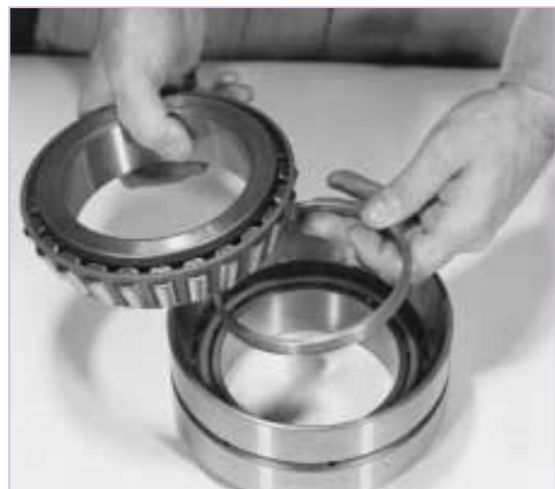
Fig. 4-17 TDO spacers This photo shows what a type TDO spacer bearing looks like. The left hand is holding a spacer which fits between the two single inner races.
