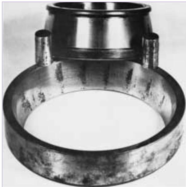
Fig. 6-9 Etching in the initial stage Pitting caused by moisture at the roller/raceway contact line.
