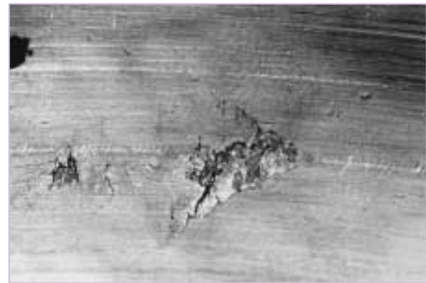
Fig. 6-2 Point Surface Origin (PSO) PSO is fatigue damage that has its origin associated with surface asperities, which act as local stress concentrations.
