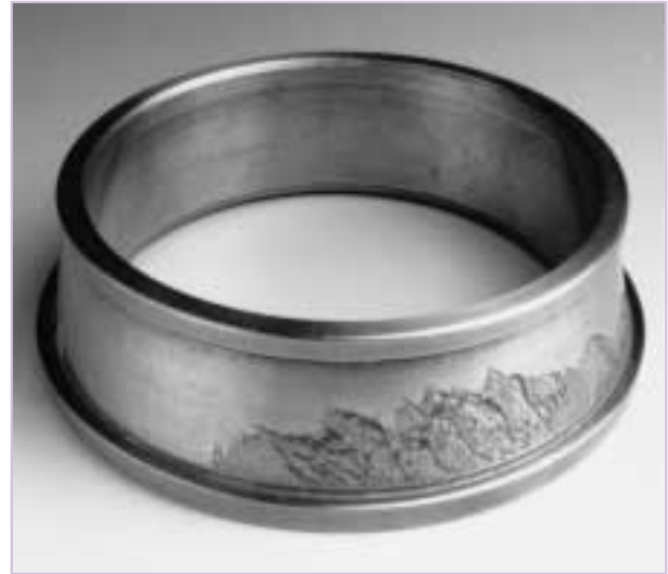
Fig. 6-1 Geometric stress concentration Geometric stress concentration fatigue results from locally increased stress at the ends of roller/race contact.
